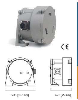
The model IT9101 is a rugged and simple device which provides a voltage divider feedback signal for incline position up to 240 degrees. The heart of the IT9101 is a magnetically-damped pendulum coupled to a conductive plastic precision potentiometer.
