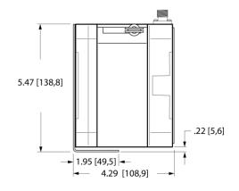
DIMENSIONS ARE IN INCHES [MM] tolerances are 0.04 IN. [1,0 MM] unless otherwise noted.
