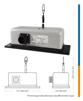
The DV301 is a combination position and velocity transducer for full-scale measurement ranges from 2 to 100 inches. A precision plastic-hybrid potentiometer provides accurate position feedback while a self-generating DC tachometer provides a velocity signal that is proportional to the speed of the traveling stainless-steel measuring cable.
