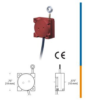
Introducing the world's smallest stringpot. The M150 is smaller than a thumbprint and occupies a tiny space of only .74 x .74 x .38 inches. With a full stroke measurement range of 1.5 inches, the M150 has been designed for many aerospace and automotive space-critical test applications such as throttle position and crash-test instrumentation.
