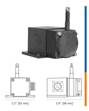
The PT1232, part of our compact line of cable extension transducers, delivers position feedback via RS232 serial communication to your data acquisition or controller system. The PT1232 sends a raw 16-bit position count from 0000 to FFFF (hex). Additionally this device can be set to continuously send data or send data only when polled.
