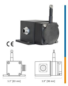
The PT1A is perfect where space and money are limited. The PT1A is part of Celesco's compact line of cable-extension transducers. Using a high cycle plastic-hybrid potentiometer, the PT1A provides a precision voltage divider position feedback signal for fullscale measurement ranges from 2 to 50 inches.
