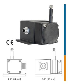
The PT1DC can operate from an unregulated 14.5 to 40 VDC power supply while providing an output signal that is proportional to the linear movement of its measuring cable. The PT1DC has a maximum measurement range up to 50" and has 4 output signal options to choose from: 0...10, 0...5, -10...+10 and -5...+5 Vdc.
