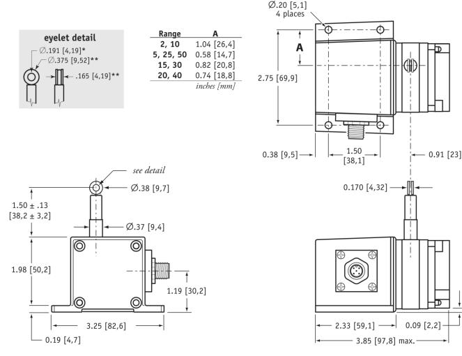
DIMENSIONS ARE IN INCHES [MM] tolerances are 0.03 IN. [0.5 MM] unless otherwise noted.
