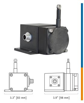
The PT1DN communicates to your PLC over DeviceNET<sup>®</sup> and provides a precision position feedback signal for full-scale measurement ranges from 2 to 50 inches. Because the PT1DN uses a potentiometer as its sensing element, the position signal is "absolute" and does not have to be reset to a "home" position upon startup.
