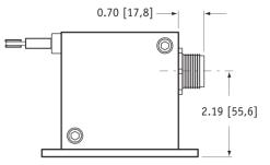
\* tolerance = +.005 -.001 [+.13 -.03] \*\* tolerance = +.005 -.005 [+.13 -.13]
