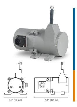
The PT8CN, using a high cycle plastic-hybrid potentiometer, communicates to your PLC via the CANbus SAE J1939 interface. Suitable for factory and harsh environment applications requiring linear position feedback in ranges up to 60".
